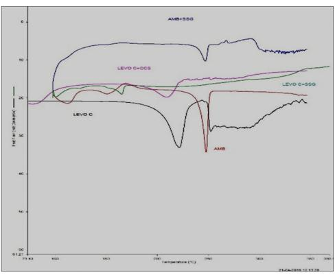
Fig. 2: Differential scanning calorimetry study of all drug mixture
