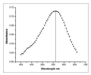
Fig. 2: Absorption maximum of 4-nitro-2-phenoxy aniline at 560 nm
