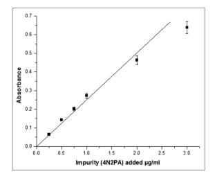
Fig. 4: Beer's law range - standard addition of 4-nitro-2-phenoxy aniline as impurity to nimesulide tablet formulations. A fixed concentration of 20 ppm of tablet solution is used to which varying amounts of 4N2PA aniline added as impurity
