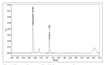
Fig. 6: Ultra performance liquid chromatography chromatogram for limit of detection of grazoprevir and elbasvir
