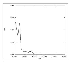
Fig. 4: Ultraviolet-visible spectrum of purified compound from Eleutherine bulbosa
