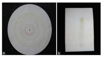
Fig. 3: (a) Circular chromatogram, (b) Thin-layer chromatogram of flower extracts of *Millingtonia hortensis* sprayed with Cu (II) – ninhydrin reagent
