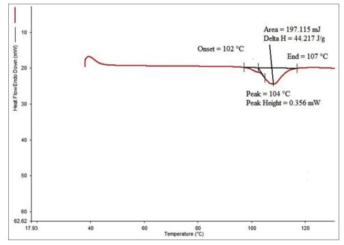
Fig. 1: Differential scanning calorimetric thermogram of tazarotene pure drug
