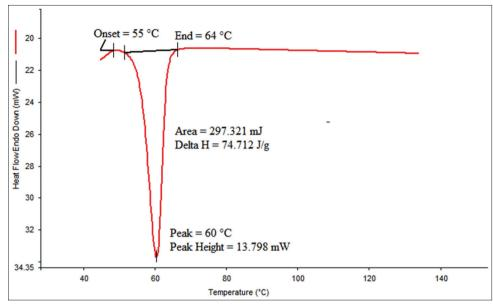
Fig. 17: Differential scanning calorimetric thermogram of tazarotene nanoformulation
