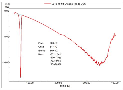
Fig. 15: Differential scanning calorimetric thermogram of dynasan-116
