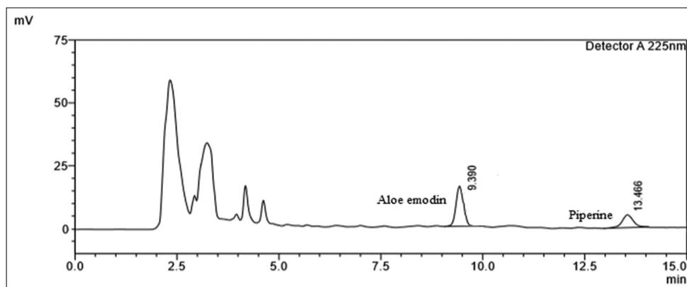
Fig. 3: High-performance liquid chromatographic chromatogram of sample mixture of aloe-emodin and piperine obtained using optimized conditions
