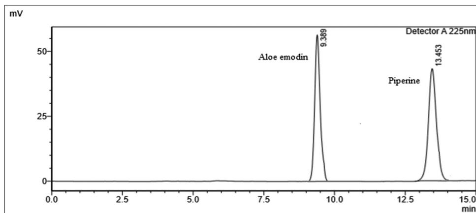
Fig. 2: High-performance liquid chromatographic chromatogram of standard mixture of aloe-emodin and piperine obtained using optimized conditions
