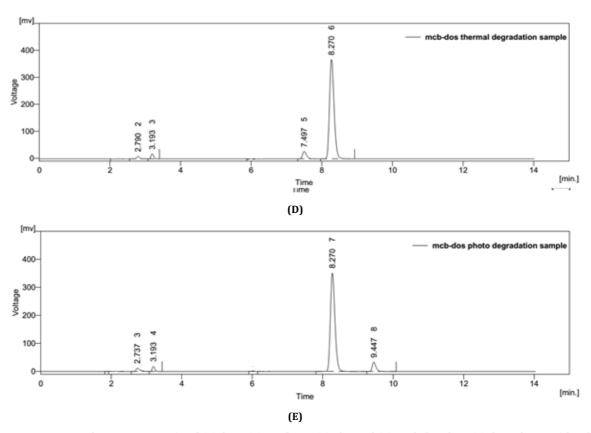
Fig. 7: Representative chromatograms of acid (A), base (B), oxidative (C), thermal (D), and photolytic (E) degradation of dosulepin hydrochloride and methylcobalamin
