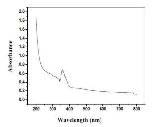
Fig. 1: UV-visible spectrum of synthesized ZnO-NPs
