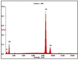
Fig. 3: EDX spectrum of synthesized ZnO-NPs
