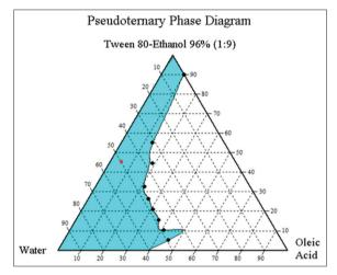
Fig. 1: Pseudoternary phase diagram of microemulsions [3]
