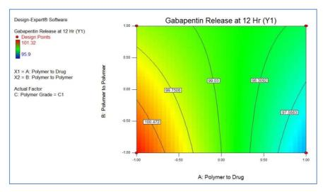
Fig. 5: Contour plot demonstrating the influence of polymer content-to-drug proportion (X1) and polymer-to-polymer proportion (X2) on the percentage of GBP release at 12 h (Y1)
