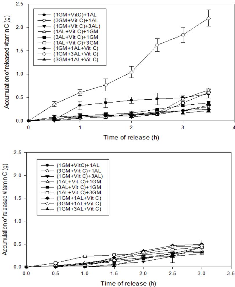
Fig. 4: Effect of encapsulation method of vitamin C on the release profile of vitamin C at pH 1.2 (top) and pH 6.8 (bottom), \*Results are expressed as mean $\pm$ SD, n=3
