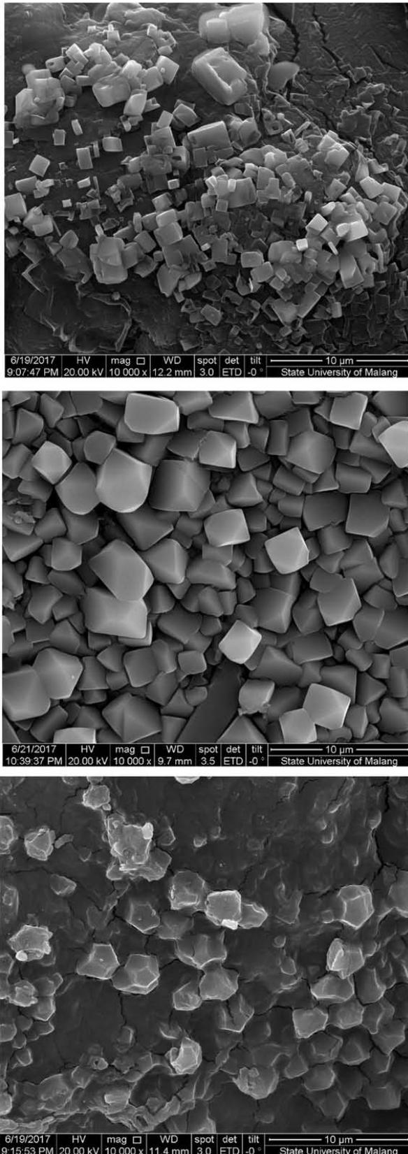
**Fig. 6: Morphology of encapsulated 3% vitamin C using various preparation methods: glucomannan and alginate (3:1, g/g) were blend together with the vitamin C (top), bead of three-parts of glucomannan and vitamin C which coated with one-part alginate (middle), bead of one part of alginate and vitamin C which coated with three-parts of glucomannan (bottom)**
