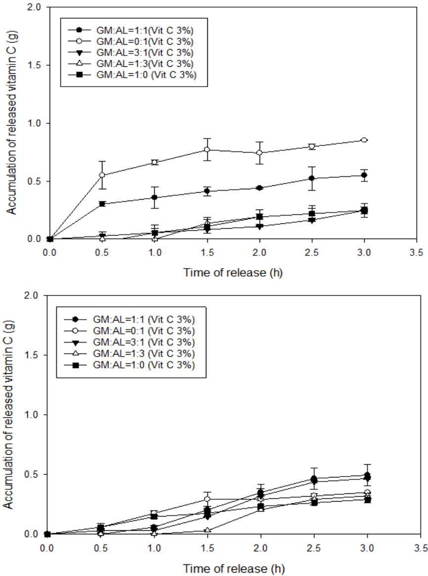
Fig. 2: Effect of various ratio of combined matrix encapsulation on the release profile of vitamin C at pH 1.2 (top) and pH 6.8 (bottom), \*results are expressed as mean±SD, n=3
