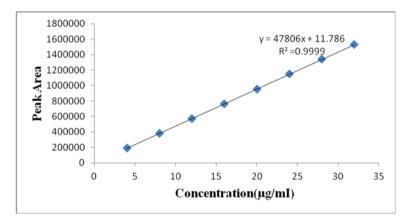
Fig. 4: Linearity plot of amlodipine besylate
