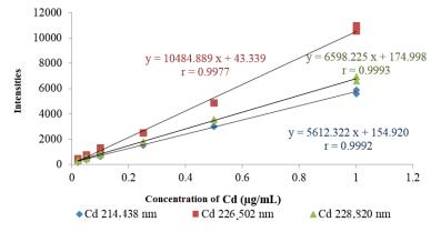
Fig. 1: The relationship between Cd concentration (x-axis) and intensity of light emitted (y-axis) at wavelengths of 214.438 nm, 226.502 nm, and 228.820 nm
