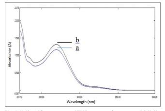
Fig. 6: Kojic acid spectrum on UV-Vis spectrophotometer: (a) Kojic acid from fermentation culture; (b) standard of kojic acid
