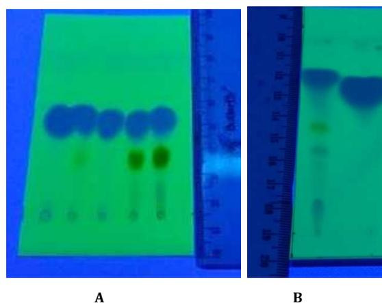
Fig. 3: TLC analysis under UV light for gamavuton-0 (Energy source: A = heating mantel and B = microwave)
