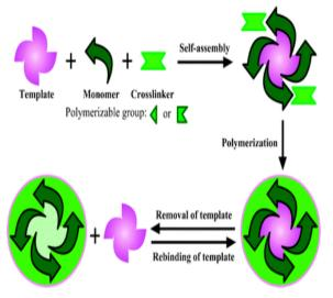
Fig. 1: Process of molecular imprinting [14]
