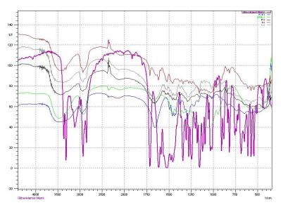
Fig. 5: FTIR spectrum of glibenclamide (purple line), PVP (blue line), HPMC (green line), F1 (black line), F10 (gray line) and F19 (brown line)
