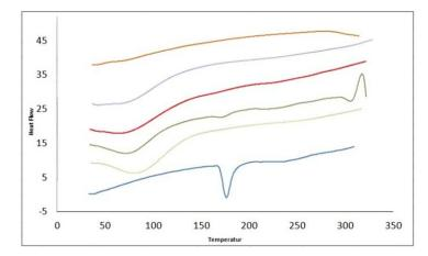
Fig. 4: DSC thermogram of glibenclamide (blue line), PVP (gray line), HPMC (green line), F1 (red line), F10 (purple line) and F19 (brown line)
