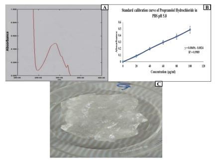
Fig. 2: (A) Lambda max of propranolol hydrochloride in PBS pH 5.8, (B) Calibration curve of propranolol hydrochloride, (C) Formulation of propranolol hydrochloride topical gel, (values are expressed as mean±standard deviation, n=3)
