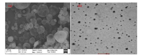
Fig. 1: SEM (a) and TEM (b) photomicrograph of optimized NLCs formulation at 1000KX
