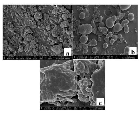
Fig. 2: Scanning electron micrograph of (a) Cu (b) Pol 407 (c) Cu-SD
