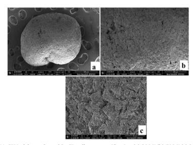
Fig. 11: SEM of the surface of Cu-SD pellet at magnification (a) 200 X (b) 500 X (c) 2000 X
