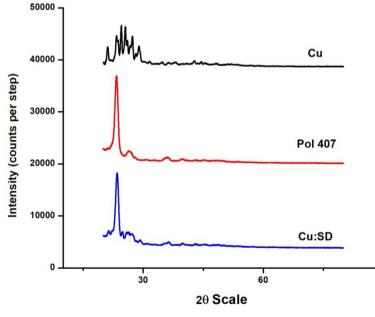
Fig. 5: XRD of (a) Cu (b) Pol 407 (c) Cu-SD
