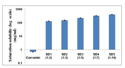
Fig. 6: Saturation solubility (mg/ml) (log scale) of Cu and Cu-SD in 0.1 N HCL, \*error bars represent standard deviations of three replicates
