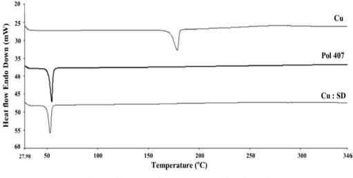
Fig. 4: Differential scanning calorimetry of (a) Cu (b) Pol 407 (c) Cu-SD
