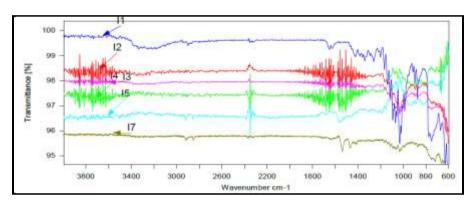
Fig. 1(B): Overlay spectra of ISDNwith all excipients, (I1 = ISDN, I2 = ISDN+MCCPH102, I3 = ISDN+HPMC K100M, I4 = ISDN+polyox<sup>tm</sup> WSR303, I4 = ISDN+HPMC K15M, I7 = ISDN+Magnesium Stearate)
