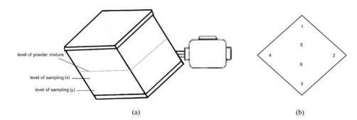
Fig. 1: Blender (a) side view presents two levels of sampling and (b) top view presents sampling positions
