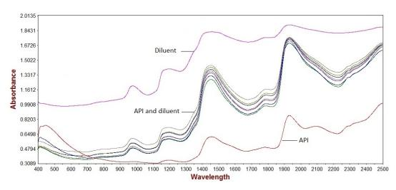
Fig. 2: NIR spectra of API, diluent and the powder blends of API and diluents
