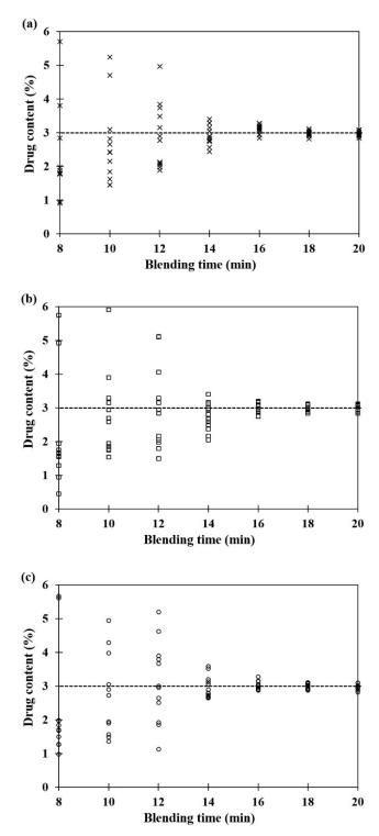
Fig. 4: The predicted API content between 8–20 min of blending process of (a) batch no. I, (b) batch no. II and (c) batch no. III (12 samples from each of the 12 locations), dot line represents the nominal API content (3%)
