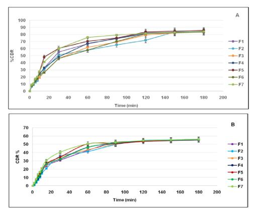
Fig.5: Percent drug release curve for F1-F7 ODF formulations in [A] phosphate buffer pH 6.8 and [B] 0.1N HCl(mean±SD; n=3)
