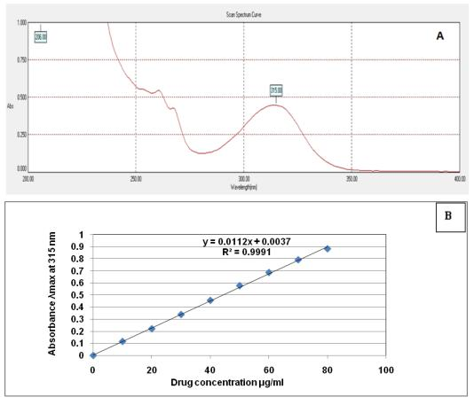
Fig.3: [A] UV scan of LH (10 µg/ml) in methanol. [B] Calibration curve of LH in methanol (mean±SD; n=3)
