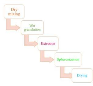
Fig. 4: Steps involved in manufacturing of pellets
