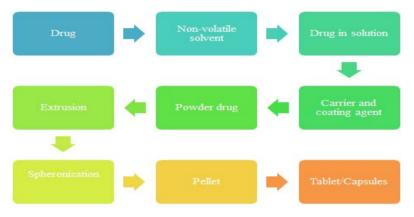
Fig. 3: Manufacturing steps involved in liquisolid-pellet technology
