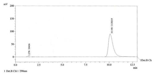
Fig. 1: Chromatogram of Sildenafil standard solution
