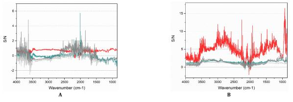
Fig. 2: Examples of S/N spectra on each day of measurements: A-powders on day 82 from the date of production, B-powders on day 131 from the date of production (red-sample 2p, green-3p, dark gray-4p, gray-5p), n=6
