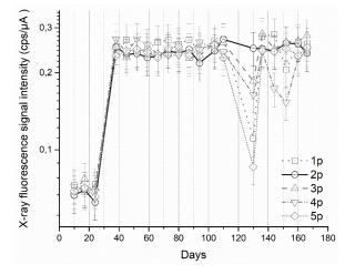
Fig. 6: Kinetics of changes in the intensity of X-ray fluorescence in the studied samples of powders at the wavelength of Kα 3.313 keV (3.7424 Å), n=6
