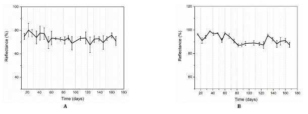
Fig. 3: Signal stability control for intact lactose-kinetics of reflection signal values at 3250 cm-1; (A-powders, B-tablets), n=6
