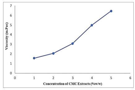
Fig. 4: Viscosity of carboxymethyl cellulose extracts (carboxymethyl cellulose from rice husk) in difference concentration
