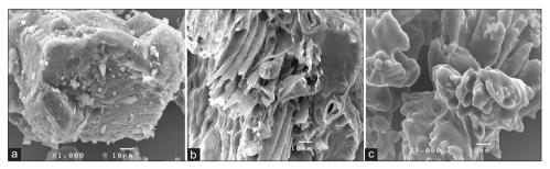
Fig. 5: Image of surface of rice husk (a), extracted cellulose (b), and extracted carboxymethyl cellulose (c) by scanning electron (magnification ×1000)
