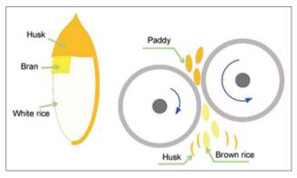
Fig. 1: The rice mill process [1]
