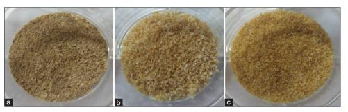
Fig. 3: Characteristics of rice husk (a), cellulose extracts (b) and carboxymethyl cellulose extracts (carboxymethyl cellulose from rice husk) (c)
