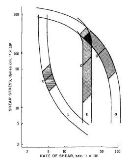
Fig. 2: A combination of master curves for lipophilic (L) and hydrophilic gels (G) and oil-in-water emulsions show the most acceptable viscosity range for spreading on the skin (shaded area) and optimal viscosity value (line 0) [2]
