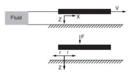
Fig. 1: Schematic representation of finger geometry as two parallel plates. V-finger velocity, Z-sample layer thickness, Xshear stress, F-shear force between fingers, R-finger radius [15]
