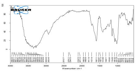
Fig. 2: FTIR spectra of starch glycolate
