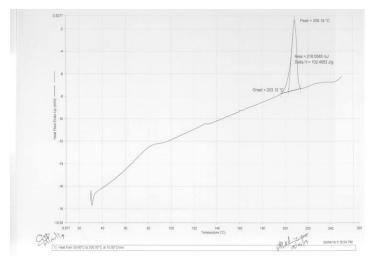
Fig. 5: DSC thermogram of glipizide with starch glycolate
