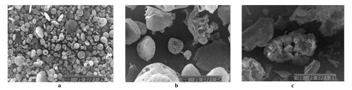
Fig. 1: Microparticles containing beetroot extract using concentration of EC 5% (a), 10% (b) and 20% (c)
