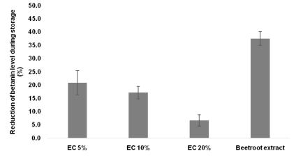
Fig. 2: Percentage reduction of betanin level during 28 d storage in microparticle EC 5%, 10%, 20% and dry beetroot extract (at 40±2 °C, RH 75%±5%). Values represent mean±SD (n=3)
