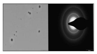
Fig. 3: TEM analysis of Selenium nanoparticles reveled size of particles 7-48 nm
