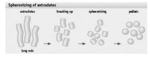
Mechanism of pellet formation by extrusion spheronization [14]
