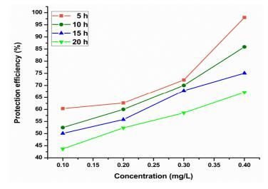
Fig. 1: Protection efficiency values obtained from weight loss technique
