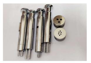
Fig. 1: It shows upper and lower multi-tip punches and die (with 3 and 5) tooling
