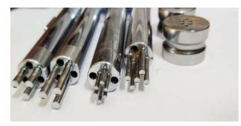
Fig. 2: It shows tip sizes of the multi tip punches/compression
