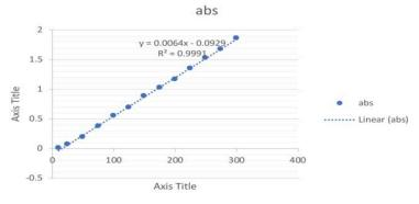
Fig. 4: Calibration curve of sitagliptin
