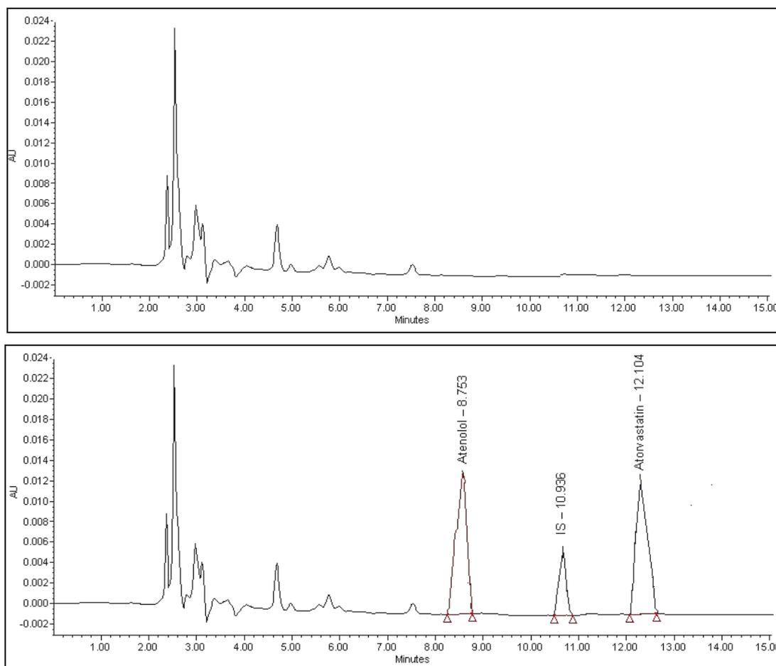
Fig. 3: Chromatogram of a) blank (ATV, ATL, and I. S. free rabbit plasma) b) plasma spiked with ATV, ATL, and I. S
