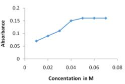
Fig. 5: Effect of concentration of 1, 10 phenanthroline on absorbance of developed system
