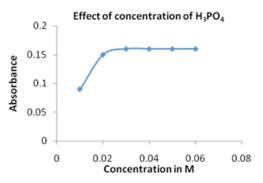
Fig. 4: Effect of concentration of H<sub>3</sub>PO<sub>4</sub> on colour development
