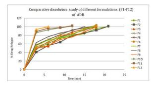
Fig. 2: Comparative *In vitro* dissolution study of mouth dissolving tablets for amlodipine besylate at 237 nm
