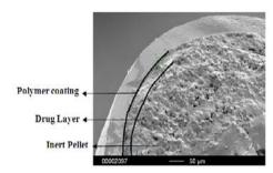
Fig. 5: SEM picture of cross section of a Taste masked pellets coated with 25 mg Eudragit EPO
