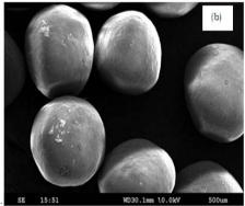
Fig. 4: SEM pictures of Taste masked pellets with a) 18.75 mg and b) 25 mg Eudragit EPO
