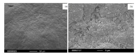
Fig. 3: SEM pictures of a) MCC pellets and b) Sugar pellets
