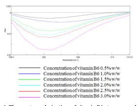
Fig. 6: The spectrum derivatives of vitamin B6 at wave number  $1280.5\text{-}1315.21\ \text{cm}^{\text{-}1}$
