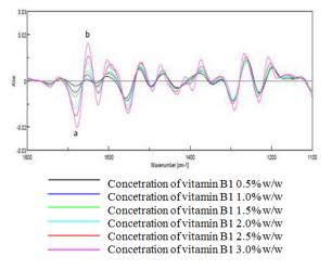
Fig. 2: The overlaid of a series concentration of vitamin B1 spectra derivatives with noted at wave numbers: (a) 1662.34-1700.91 cm<sup>-1</sup> and (b) 1646.91-1662.34 cm<sup>-1</sup>
