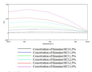
Fig. 3: Vitamin B1 spectra derivatives at wave numbers 1646.91–1662.34  $\rm cm^{-1}$
