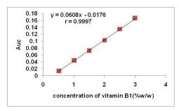
Fig. 7: Calibration curve of standard vitamin B1 against the area under curve of absorbance derivate
