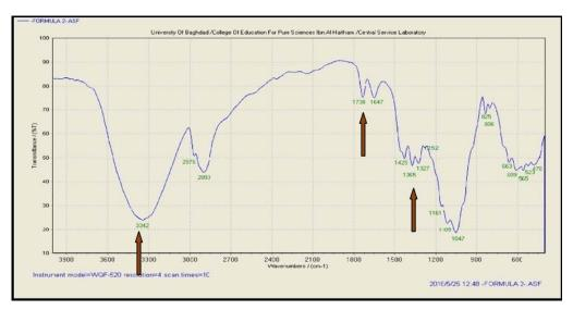
Fig. 6: FT-IR Spectrum of the liquisolid formula F11
