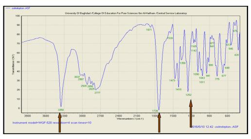
Fig. 5: FT-IR spectrum of pure zolmitriptan
