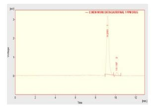
Fig. 10: HPLC Chromatogram of Nimodipine
