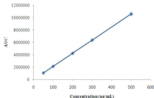
**Fig. 1: Calibration curve of hydroxychavicol standard**
