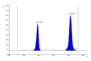
Fig. 2: Densitogram obtained from mixed standard solution of ROS and FEN scanned at 246 nm.
