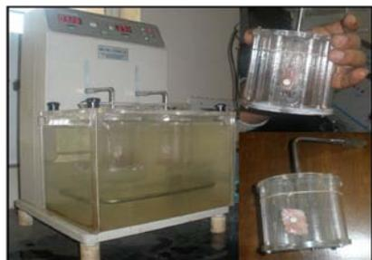
Fig. 2: Disintegration test apparatus
