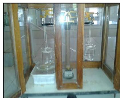
**Fig. 1: Modified physical double beam balance**
