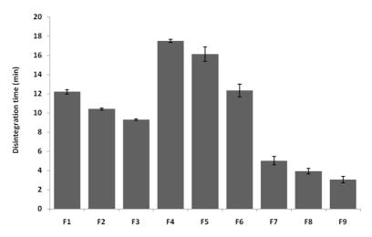
Fig. 4: Graph of disintegration time of different tablet formulations (n=3, data presented as mean±SEM. F1=formulation containing 2% chitosan, F2=formulation containing 4% chitosan, F3=formulation containing 8% chitosan, F4=formulation containing 2% corn starch, F5=formulation containing 4% corn starch, F6=formulation containing 8% corn starch, F7=formulation containing 2% Ac-Di-Sol®, F8=formulation containing 4% Ac-Di-Sol®, F9=formulation containing 8% Ac-Di-Sol®)
