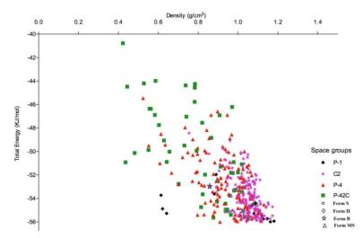
Fig. 7: Crystal energy landscape within 16KJ/mol of global energy minimum. The lattice energy minima corresponding to the experimental crystal structure are also shown
