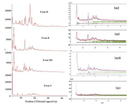
Fig. 2: PXRD pattern of polymorphs of nateglinide and their comparison with the respective simulated pattern (black line indicates the difference between the experimental and simulated PXRD pattern
