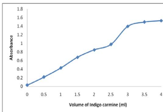
Fig. 5: Effect of variation of volume of Indigo carmine dye on the absorbance at 660 nm.
