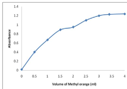
Fig. 4: Effect of variation of volume of Methyl orange dye on the absorbance at 507 nm.
