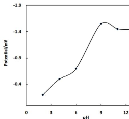
Fig. 4: The plot of the potential vs pH of DLTD in PB solution, concentration:  $2.55 \times 10^{-5}$  M at glassy carbon electrode in different pH values.
